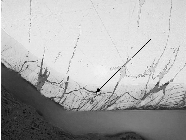
Fig. 3 – Layer microstructure in 1.4922 steel with typical horizontal cracks (magnified 500x)
