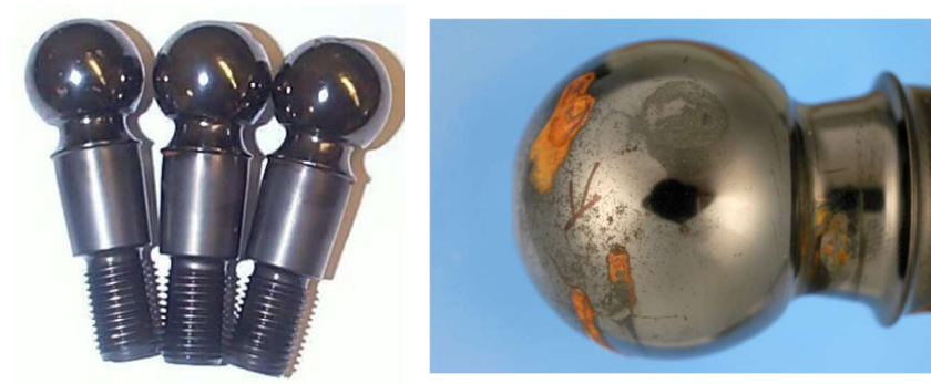
Fig. 2 – The example of Corr-I-dur® application on ball pins before and after corrosion test.
